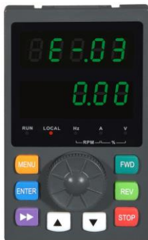
Fig. 4-5 Fault alarm display state
